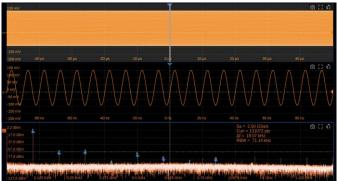
FFT supports up to 8 Mpts operation. This provides high-frequency resolution with a fast refresh rate. The FFT function also supports a variety of window functions so that it can adapt to different spectrum measurement needs. Three modes (Normal, Average, and Max hold) can satisfy different requirements for observing the power spectrum. Auto peak detection and markers are supported.
