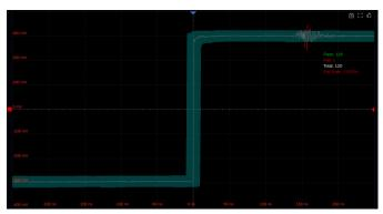
The oscilloscope utilizes a hardware-based Mask Test function, performing up to 80,000 Pass / Fail decisions each second. It is easy to generate user-defined test templates to provide trace mask comparisons, making it suitable for long-term signal monitoring or automated production line testing
